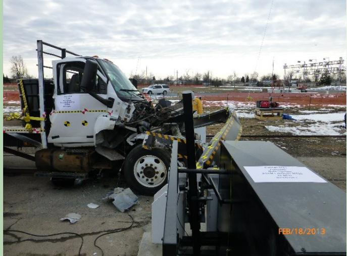
Designed and used for both perimeter high security and vehicular traffic control. Proven low maintenance, high cyclic/high volume operation, and low cost of ownership. Immobilizes vehicles weighing up to 15,000 lbs. traveling at 30 mph with under 3 feet of penetration. All systems are completely electric (no hydraulics) and are battery backed-up for hundreds of cycles in the event of AC power loss.
