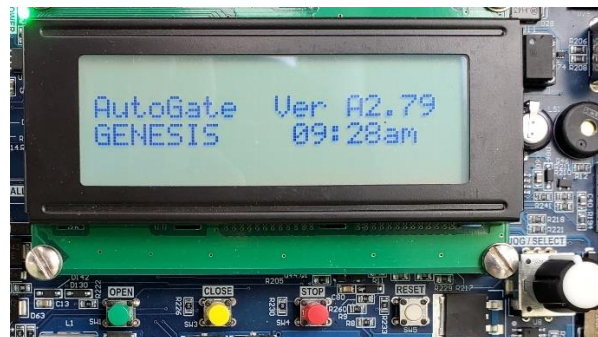
Figure 8: Image showing the location of the GREEN “Open”, YELLOW “Close”, RED Stop, Reset and Jog Select buttons on the Genesis board.
