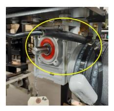
c.) Use the (2) 24.0" Cable Ties to secure the Heat Tape in place by tightening them in a cross "X" position. (Making sure to locate the Heat Tape End <u>HIGH</u> above the Shaft from the motor to prevent binding. You will secure it when you wrap the Foil Insulation around it.)
