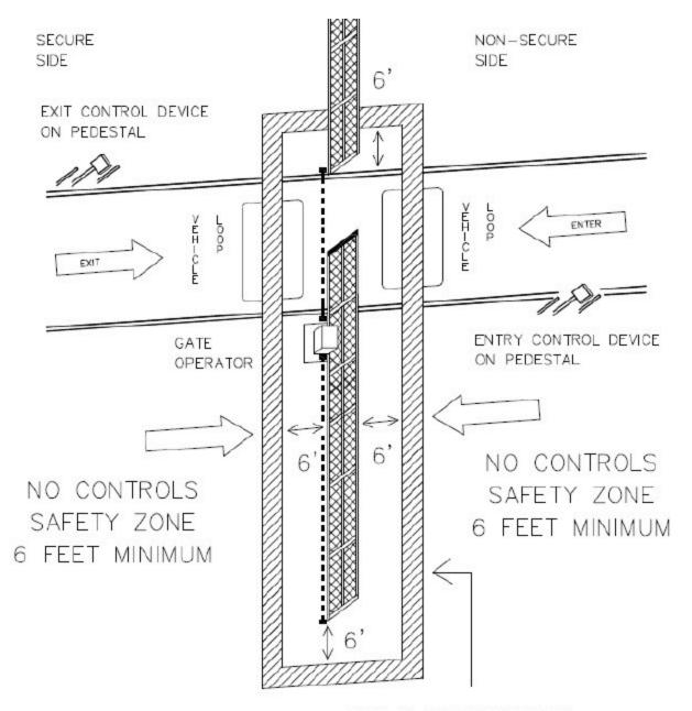
AREA OF STATIONARY FENCE COVERED BY MOVING GATE PANEL WHEN IN THE OPEN POSITION
