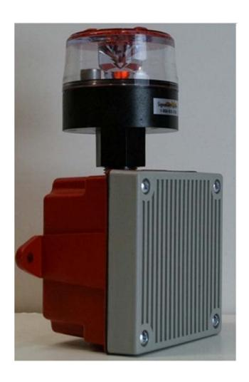
The above device, with visual signals available in red or amber lens options utilize an electronic horn to produce an attention grabbing alarm tone. The visual signal portion incorporates a strobe LED light source in a flashing pattern. Available operating voltage options are either 120 volt AC, or the DC unit that will operate at 12 or 24 volt DC. A cast zinc weatherproof back box encases the horn electronics, and accommodates mounting of the visual signal.
